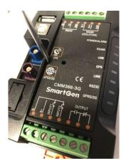
Once open you will see the SIM Card bracket. To unlock the bracket simply slide the small metal lock down gently. You should then be able to lift the bracket once unlocked. Slide the SIM Card into the bracket ensuring that it is orientated correctly.
