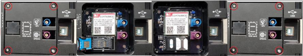
Fig. 14 SIM Card Installation Method
