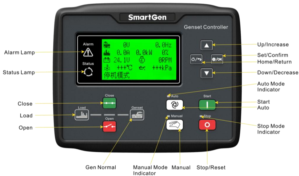
Fig.1 - HGM6110N/ HGM6110NC/ HGM6110CAN Front Panel Indication
